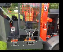
Ergonomic operator safety station with 4-way Joysticks
